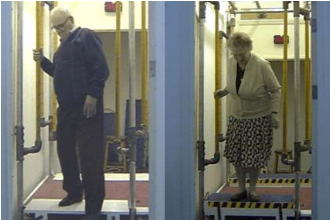
Figure 3: Extracts from video clips for two individuals leaving the vehicle ingress/egress rig.
