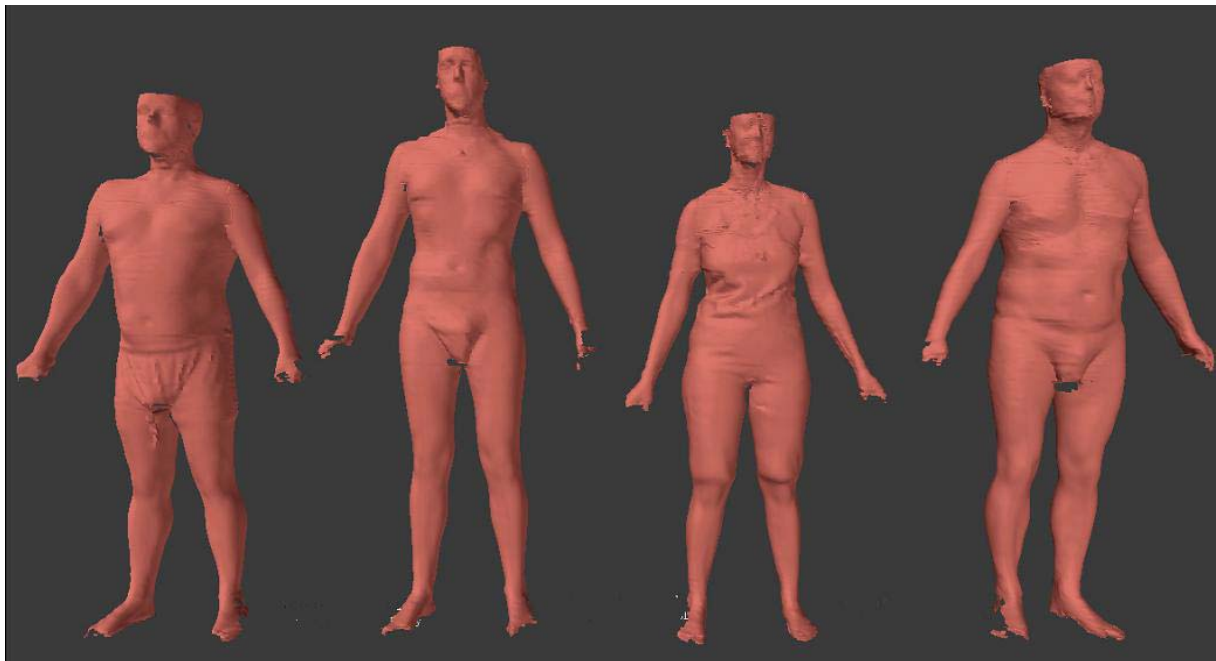
Figure 1: Scanned images for individuals that are used to collect anthropometric data and to construct the matching SAMMIE human models.
