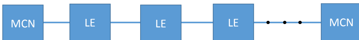
Figure 3. Horseshoe / chain architecture for current BT metro network
