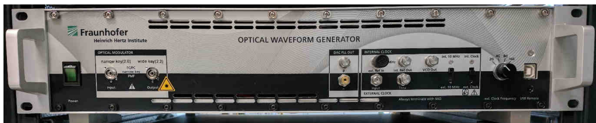
Figure 63. Optical waveform generator prototype in filterless testbed
