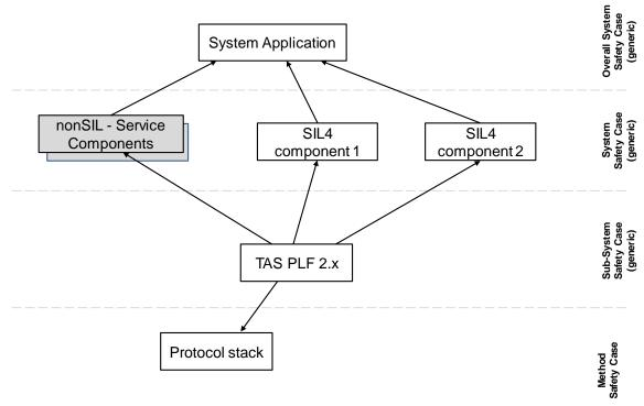
Figure 7: Hierarchical structure of the safety cases [Image: THALES].
