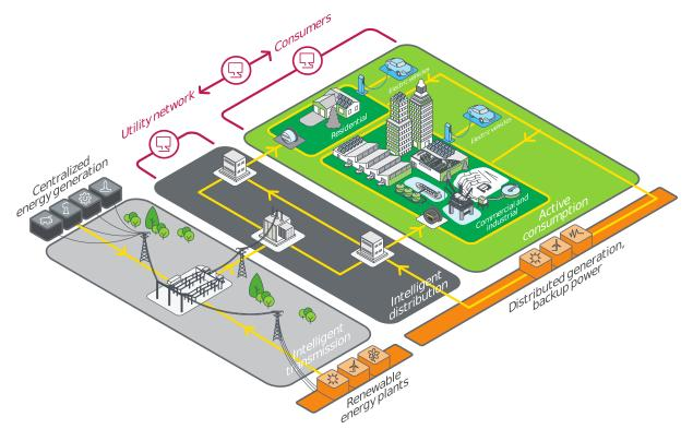
Figure 6: Components of smart grids and their interactions [Image: Schneider Electric].
