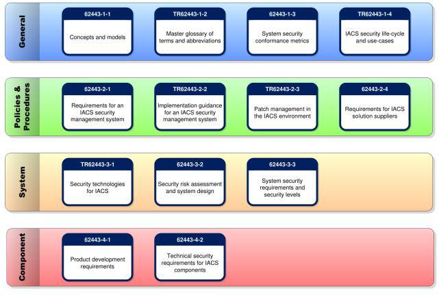
Figure 5: The elements of the IEC 62443 series. [Image: WikiMedia, CC BY-SA 3.0].
