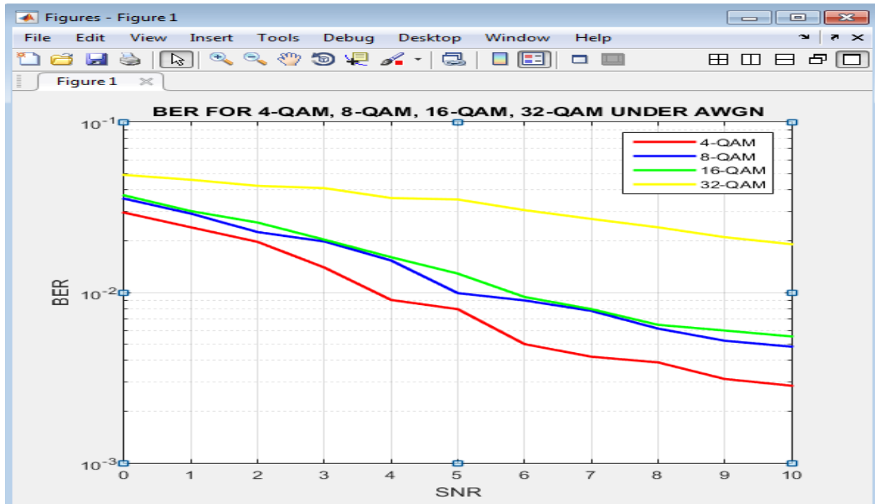
Figure 9: BER of 4-QAM, 8-QAM, 16-QAM and 32-QAM
