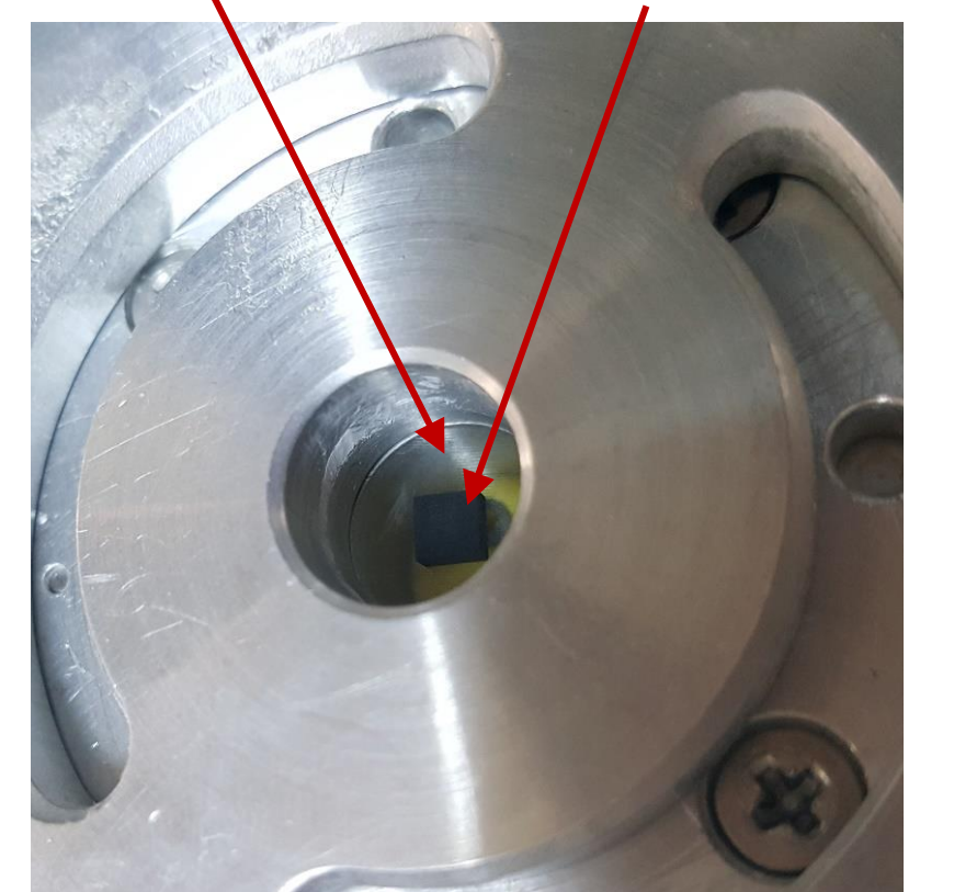
Close-up view of membrane with the attached mass
