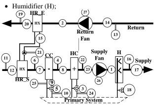
Figure 2. Schematic of the AHU under study
