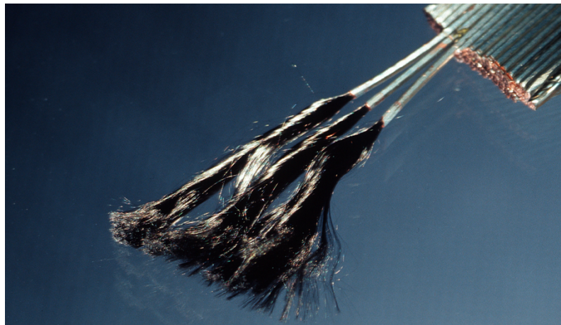
Figure 3: Superconducting Rutherford cable composed of 28 strands (Lackner 2017)
