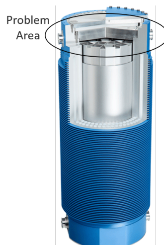
Figure 12: Illustration where the novel epoxy CTD-101K might be used for radioactive waste containment
