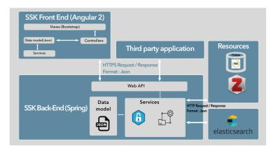
• This core/back-end communicates with a search engine, part of the architecture, based on Apache Lucene: ElasticSearch.
