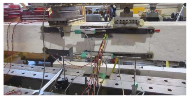
Fig. 3 LVDT setup for UHPFRC members (a) longitudinal LVDTs measuring axial deformations of slender columns (b) horizontal LVDTs measuring lateral deformations of slender columns (c) longitudinal and vertical LVDTs measuring rotations and vertical deformations of UHPFRC beam
