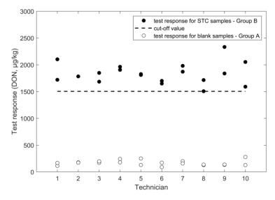
Figure 2. FPIA results for DON analysis in wheat negative and STC (1600 µg/kg) samples.
