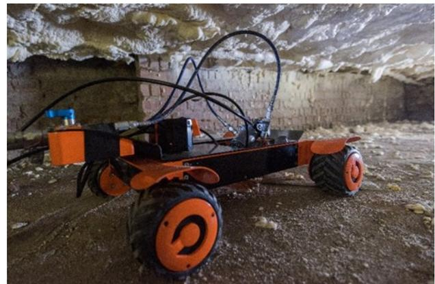
**Figure 10:** The robot after application of insulation to the underside of the floor above.
