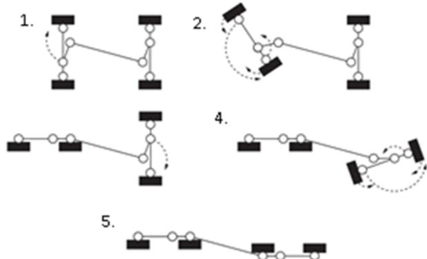
**Figure 3:** Initial proposed folding mechanism.
