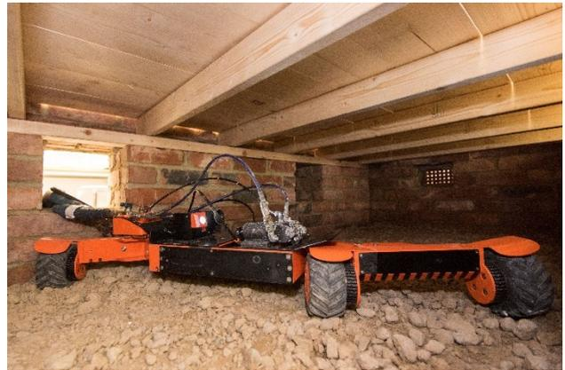
**Figure 8:** The robot in its folded position inside the void.
