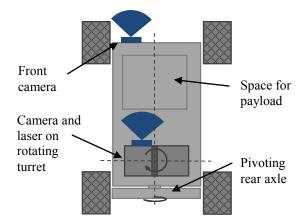
Figure 2: Top view of the robotic vehicle.
