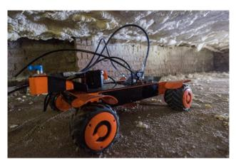
**Figure 10:** The robot after application of insulation to the underside of the floor above.
