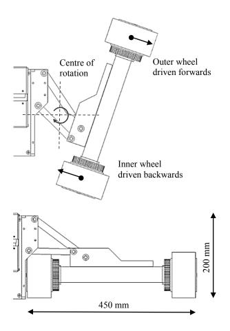
**Figure 4:** Final folding mechanism shown partially folded (top) and fully folded (bottom).
