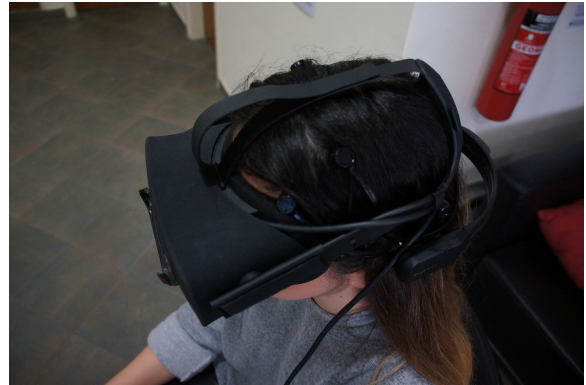
Figure 3: One of the participants wearing EMOTIV EPOC+ and Oculus Rift
