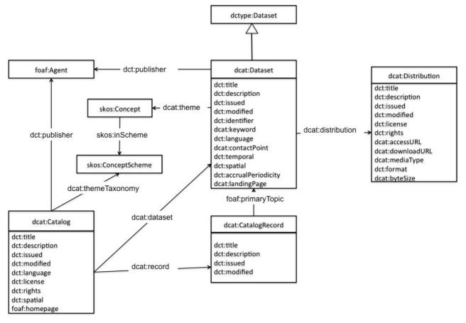
Figure 1. The DCAT data model
