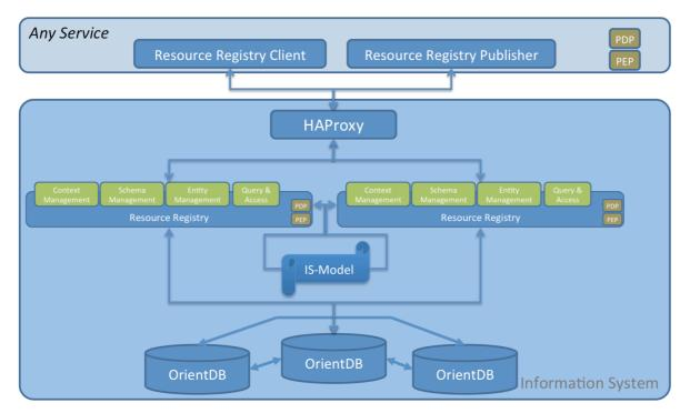
Figure 27. Joint Resource Registry Architecture
