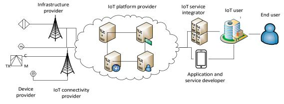
Figure 1. IoT value chain model.
