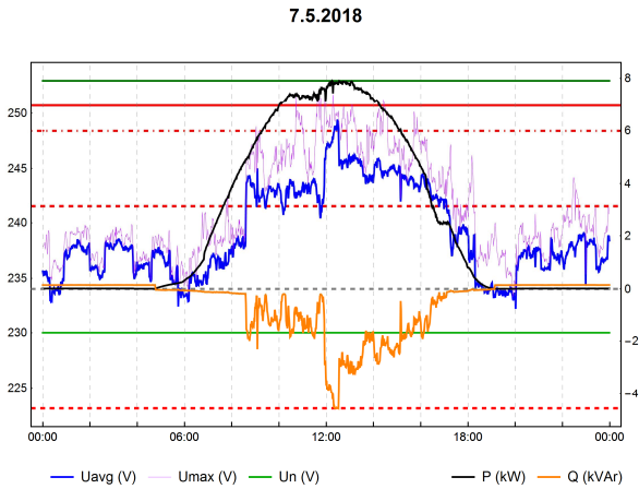
Fig. 10. Daily behavior of smart PV inverter with Q (V) and P (V) functions
