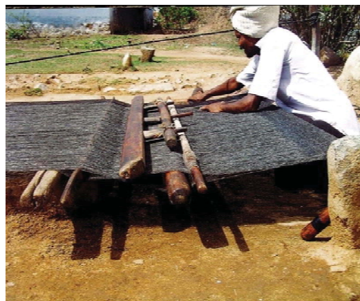
Fig. 7 Pit loom for Gongadi weaving [10]
