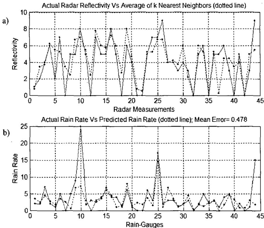
Fig. 2. An example of the input radar reflectivity pattern (red line) with the average of the matching radar patterns (blue dotted line) for the KNN system. Figure 2b shows the average of the corresponding rain patterns (red line) along with the predicted rain pattern (blue dotted line).
