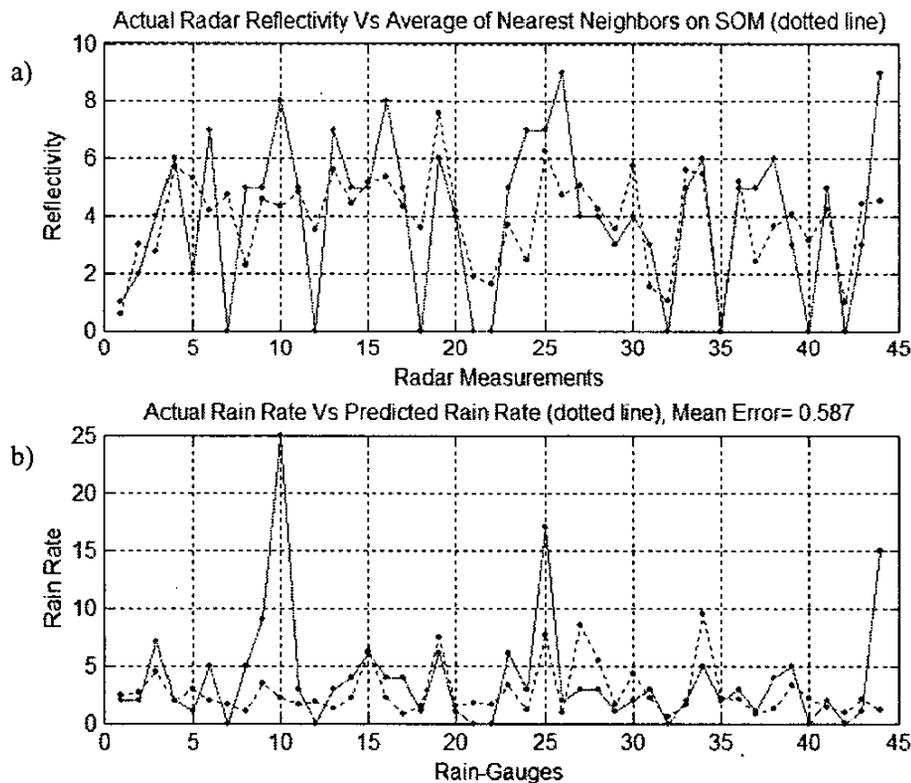
Fig. 1. An example of the input radar reflectivity pattern (red line) with the average of the matching radar patterns (blue dotted line) for the SOM system. Figure 1b shows the average of the corresponding rain patterns (red line) along with the predicted rain pattern (blue dotted line).
