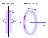
Figure 1: On the left: a vortex line with healing length  $\xi$ , actually a vortex tube. On the right: a vortex ring (vortex torus) where  $v_1$  is the toroidal velocity,  $v_2$  the poloidal velocity and  $v_3$  the translational velocity of the vortex.
