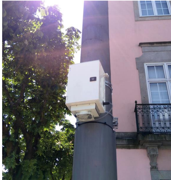
Figure 9: Air Quality sensor in Porto
