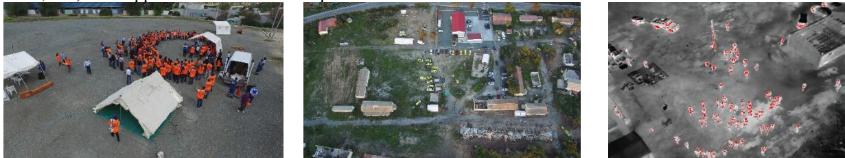
Fig. 5. Drone as future first responders can: (a) assist civil protection units in organization and planning, (b) provide situational awareness of disaster-stricken areas, (c) locate disaster survivors with thermal cameras.
