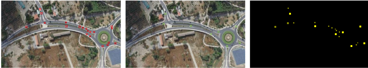
Fig. 3. Vehicle detection using drones: (a) vehicles detected using motion, (b) vehicles detected using still images, and (c) combined detection of vehicles.
