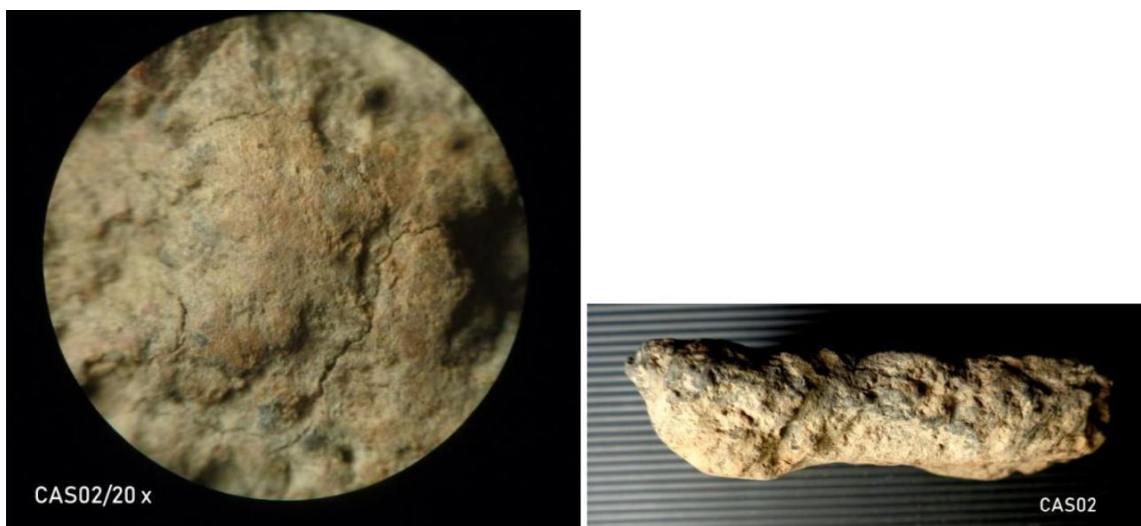
Images (008) (009): CAS02- MACRO weathering cracks on surface and cross-section
