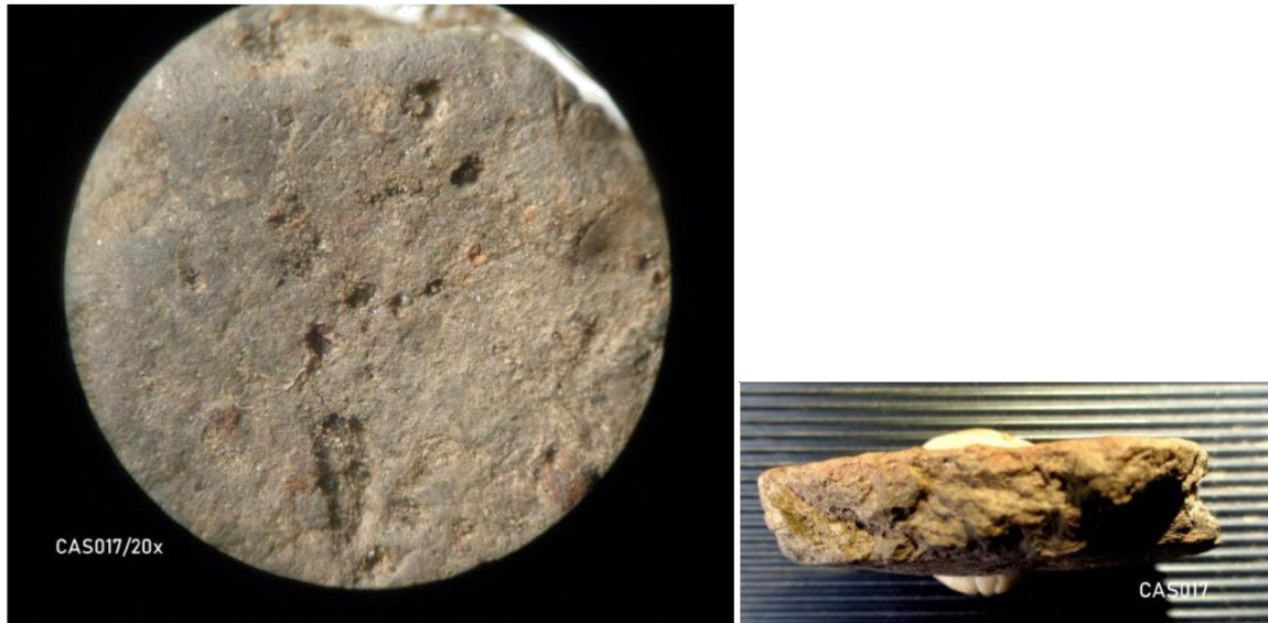
Images (068) (069): CAS017- MACRO Features of smooth black surface and cross- section
