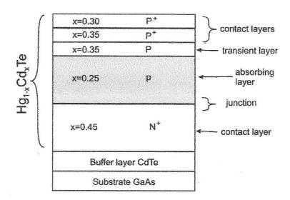
**Figure 2.** Example of the structure of HgCdTe photodiode (after [4]).
