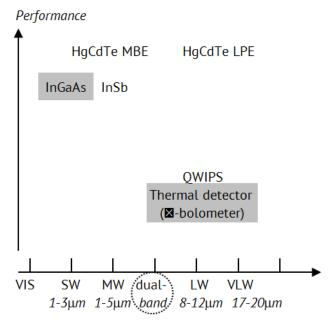
**Figure 4.** HgCdTe detectors grown by MBE and LPE deliver better object identification capability than the detectors, such as **⋈**-bolometers and those based on InGaAs and InSb = *uncooled*; all other: *cooled* (after [7]).
