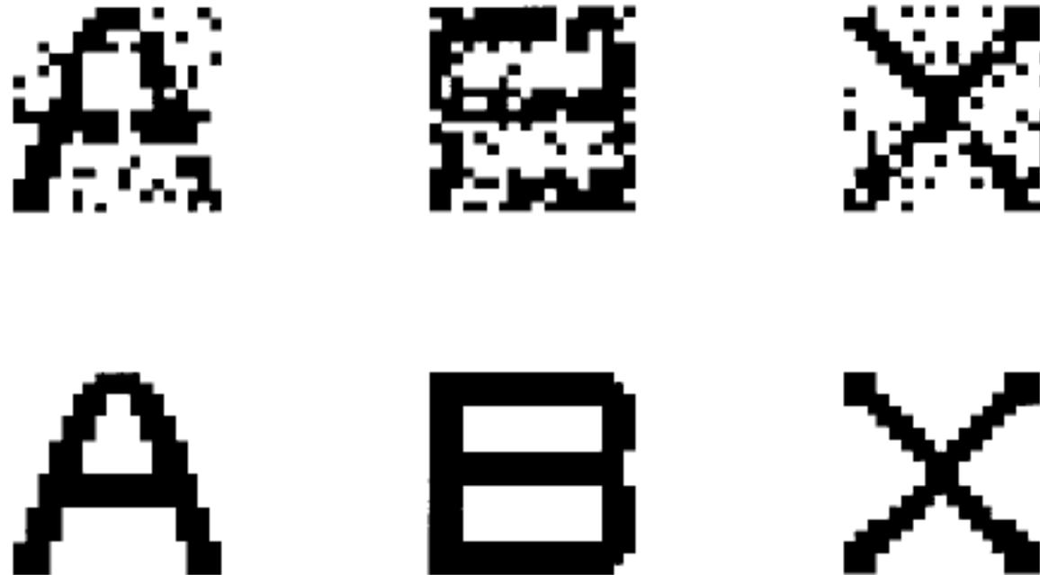
Fig. 7. An example of the behavior of the memory  $\{input \rightarrow M_{ZZ} \rightarrow W_{ZY} \rightarrow output\}$ . The memory was trained using the ten exemplars shown in Fig. 2. Presenting the memory with the corrupted patterns of the letters A, B, and X resulted in perfect recall (lower row). Each letter was corrupted by randomly reversing each bit with a probability of 0.15.
