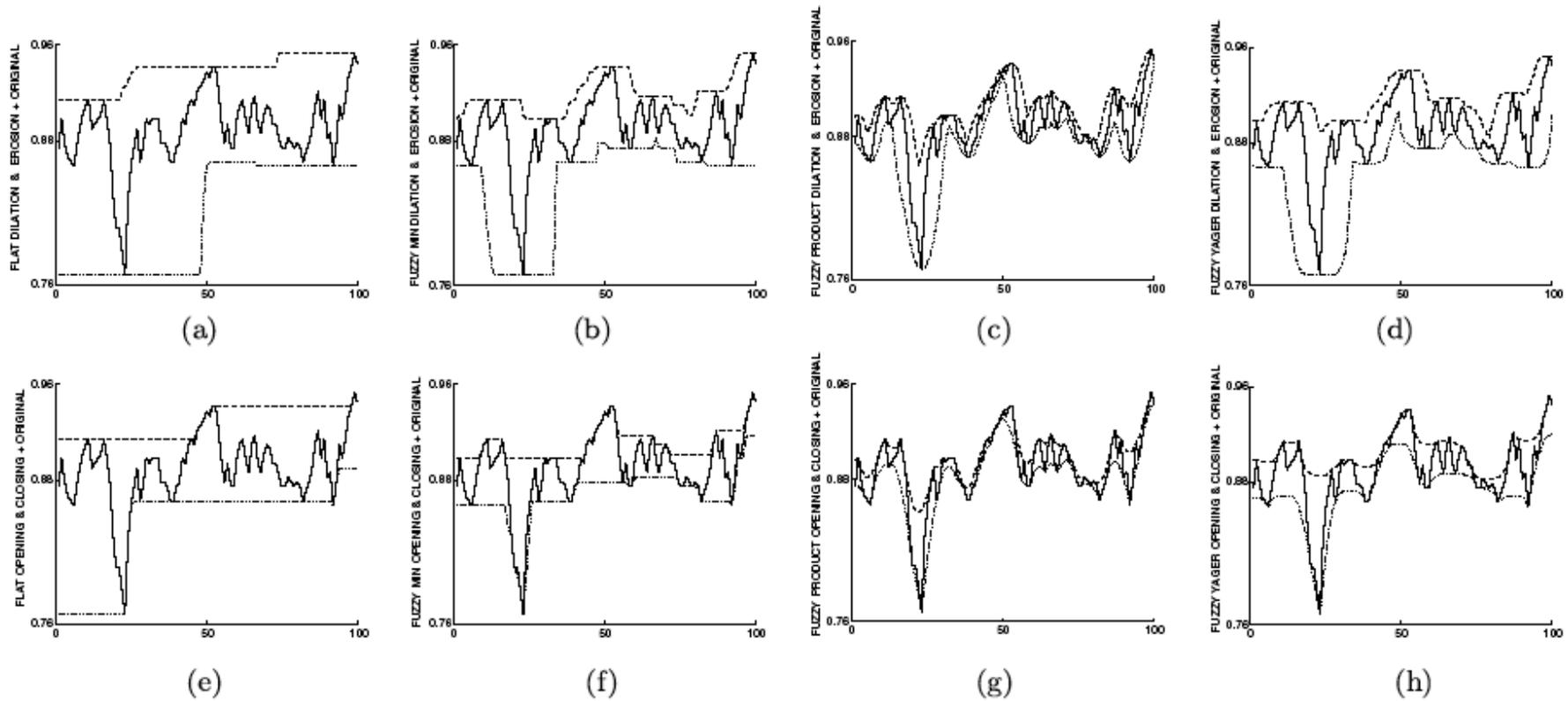
*Figure 1.* Comparison of 1D basic morphological and lattice-fuzzy signal operators. Rows 1 and 2, left to right: flat, minimum, product, Yager. Row 1: original signal (solid line), dilation (dashed line), erosion (dotted line). Row 2: closing (dashed line), opening (dotted line). Courtesy of [27].
