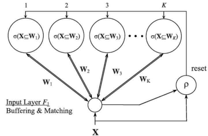
Fig. 2. flrART neural architecture for clustering, where an input pattern  $\mathbf{X}$  is in the lattice  $(\mathcal{J}_1^N, \subseteq)$  of intervals.
