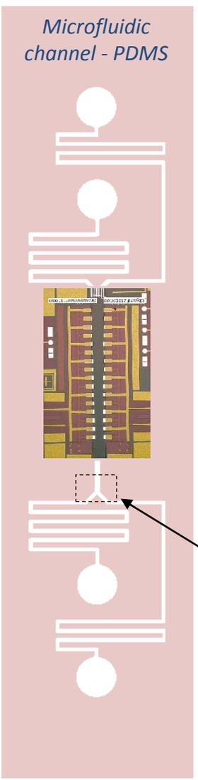
New micro channel design to ensure optimal cell location thanks to natural cell flow focusing
