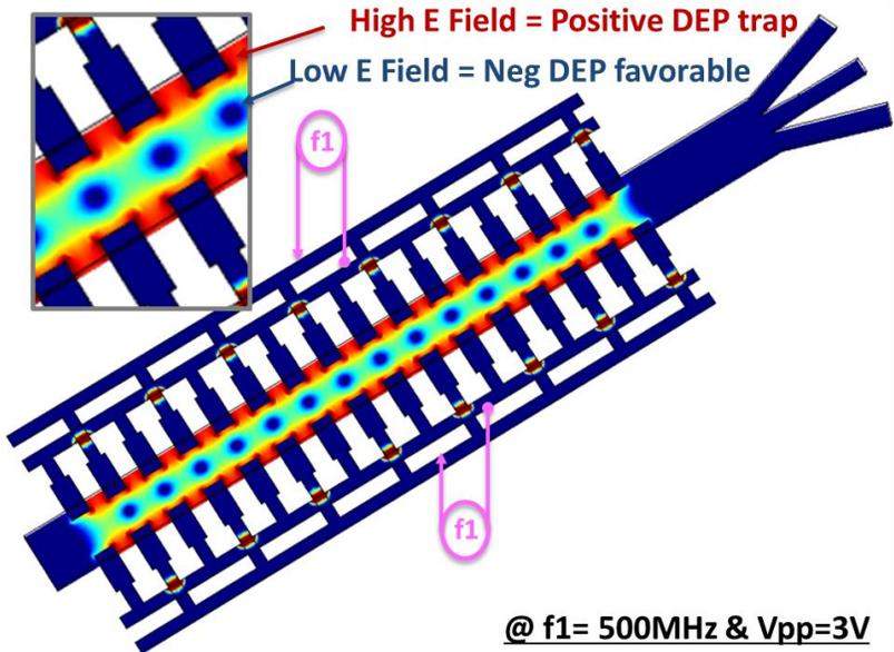
➔ EM simulations predict a suitable E field gradient distributed along the channel section
