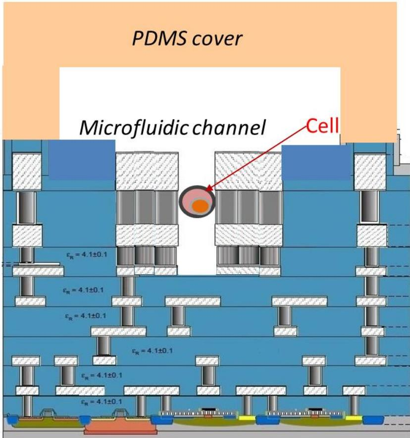
~ 9µm thick electrodes embedded in the µfluidic channel
