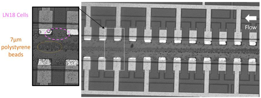
Stacked image of LN18 cells and polystyrene beads with a 50MHz DEP signal
