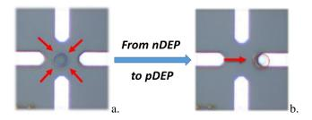
Fig. 2. DEP single cell manipulation principle – Cell Repulsion at system center with nDEP (a), Cell attraction toward electrode with pDEP (b).
