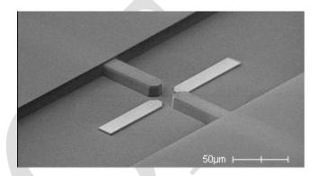
Fig. 1. Quadrupole electrodes system implemented in BiCMOS back end of line SG25H4 technology from IHP.
