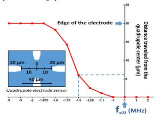
Fig. 7. Simulated cell location change from the center of the quadrupole electrodes system for different DEP signal frequency tuned around the cell crossover frequency.
