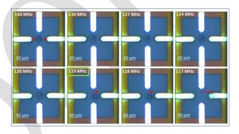
Fig. 6. Cultured in NN - Microscope imaging sequence of GBM cell crossover frequency measurement (119 MHz) by tuning the DEP signal frequency.
