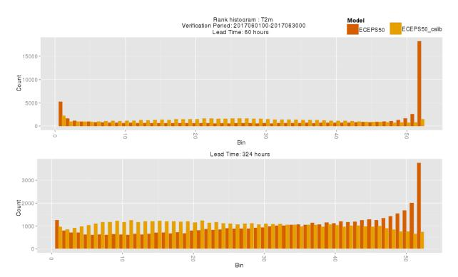
Figure 2: Rank histograms illustrating the under dispersion and negative (cold) bias of raw temperature forecasts with lead times of 60 (upper) and 324 hours (lower). (ECEPS50 = ECMWF-ENS)
