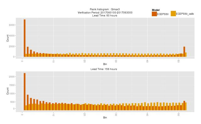
Figure 3: Rank histograms illustrating the under dispersion and positive bias of raw wind gust forecasts with lead times of 60 (upper) and 156 hours (lower). (ECEPS50 = ECMWF-ENS)
