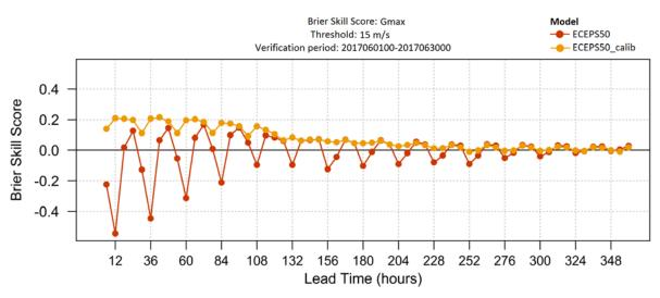
Figure 5: The Brier skill score for probabilistic wind gust forecasts (threshold 15 m/s)
