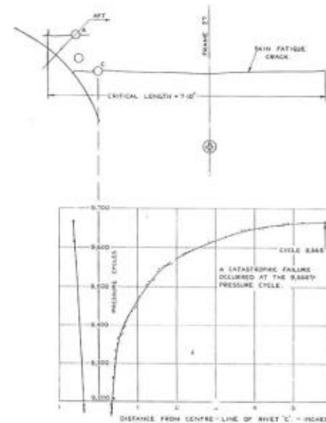
FIG. 29. Crack growth at fourth window, port side. (Top rear corner)
