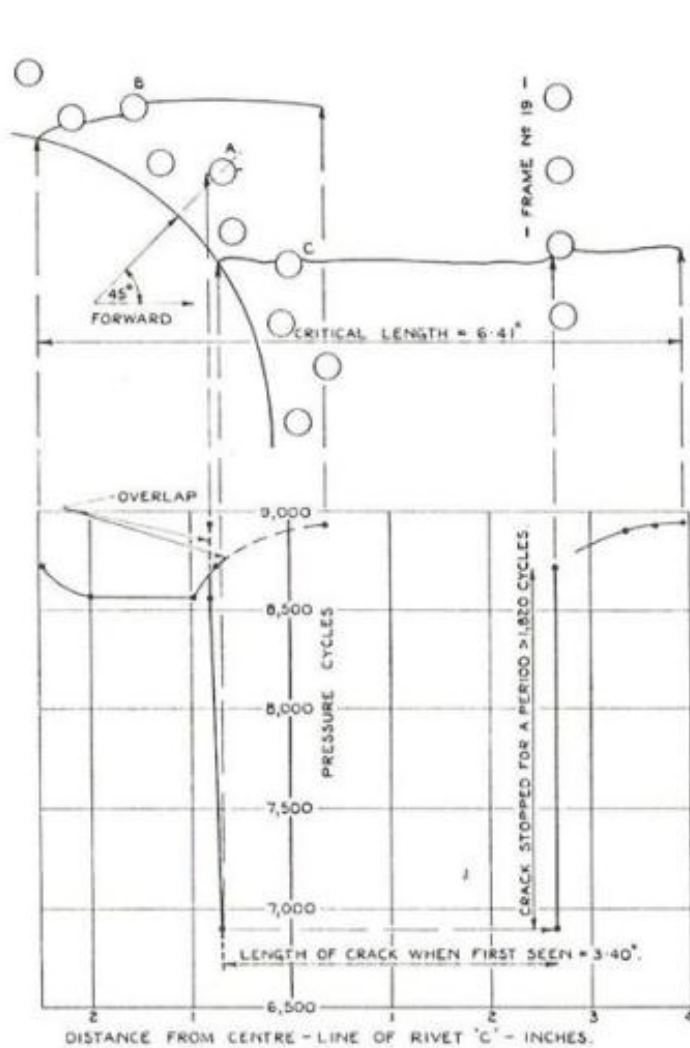
FIG. 25. Crack growth at first window, starboard side. (Top forward corner)
