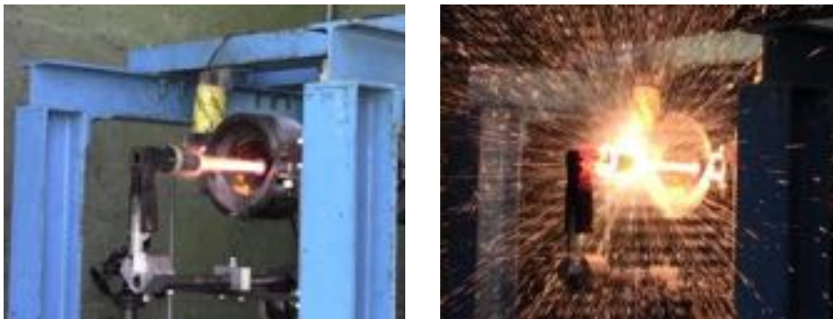
Fig. 13. Pictures of test on ZBSC-LF-2 sample, before (left) and after (right) the temperature jump (Test condition 2).
