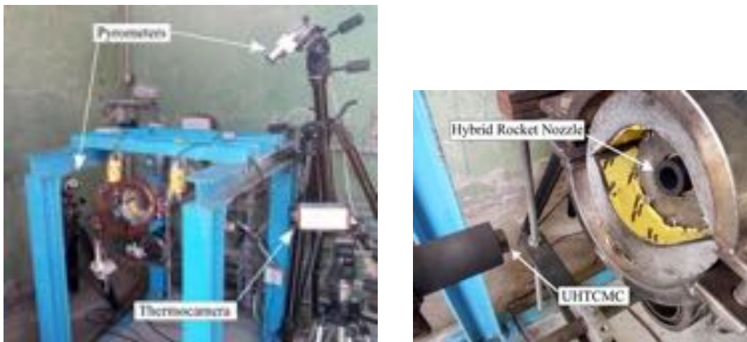
Fig. 3. Set-up for free-jet test. The area within the red circle in the left picture is zoomed in the right picture.
