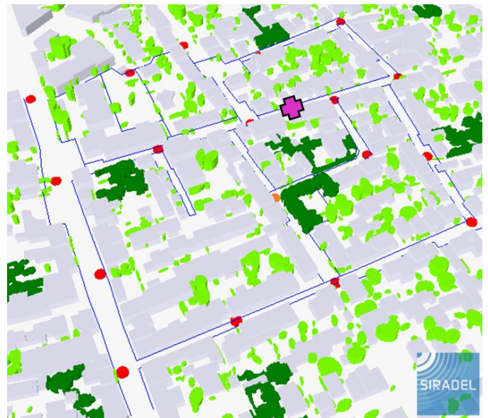
Fig. 3. Target service locations are represented by blue lines; and proposed small-deployment by red dots. The study area is 300 m × 300 m wide.
