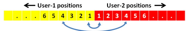
Fig. 2. User positions of two-simultaneous users separated in small steps of a wavelength in each step.
