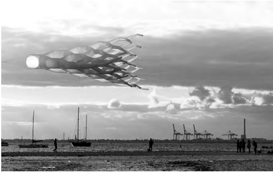
Figure 1: 12m-long self-inflating structure during a test flight. (source: Roudavski, 2017)
