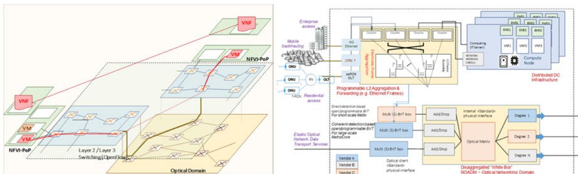
Fig. 1. Metro-Haul Infrastructure, showing the main components: the disaggregated transport network interconnecting Metro-Haul locations (AMEN/MCEN nodes), the packet switched networks and the NFVI PoP encompassing computing, storage resources.
