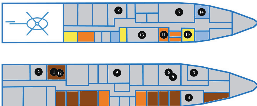
Figure 12: The ship with circadian timing has most areas under control of the dynamic light management changing the colour, intensity and direction of light. Few areas require constant lighting.
