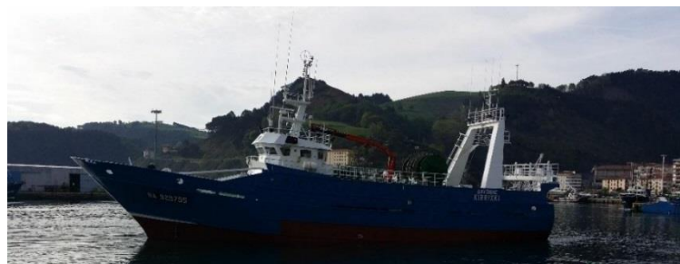
Figure 16: Typical medium sized mixed demersal bottom trawler fishing in the Bay of Biscay
