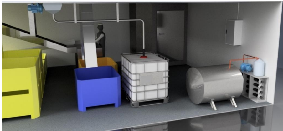
Figure 15: The setup in the storage hold, the slurry ice tank is at the right side, the IBC silage tank in the middle, the fish tubs indented for UUC and fish under MCRS on left.
