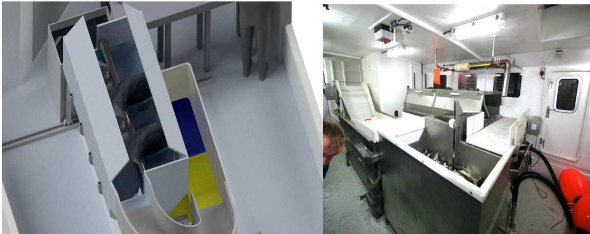
Figure 8: A visualization of the cooling above deck in Cleopatra 38 or equivalent sized vessel (left) and a real setup on a slightly larger boat, Cleopatra 50 (right).
