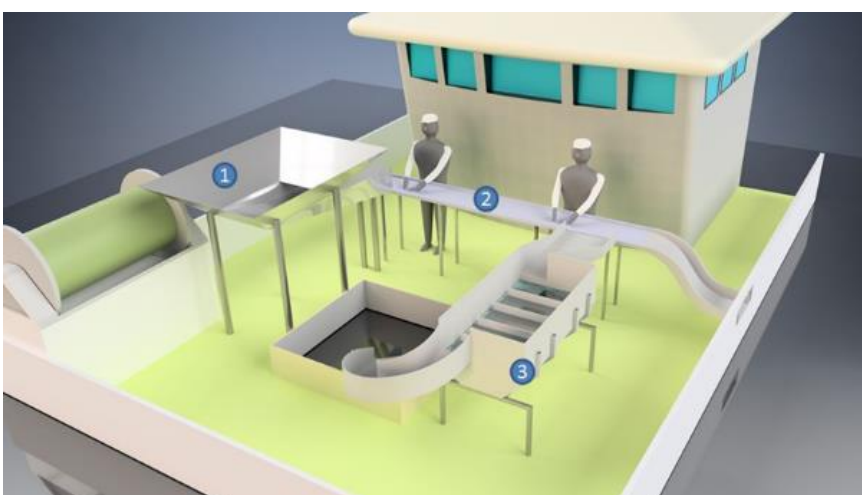
Figure 11: The upper figure shows a trawler similar to the one used for the demonstrations and the lower shows technical drawing of the current processing arrangements on board (1. Reception - 2. Bleeding and gutting - 3. Bleeding / cleaning tank)
