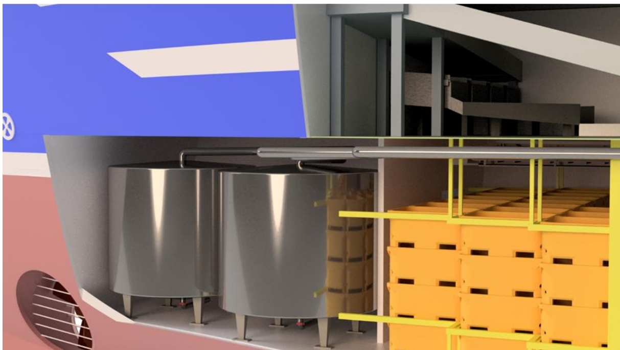
Figure 23: The primary silage tanks (top) and the storage tanks (bottom)
