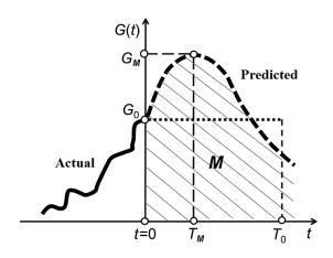
**Figure 1.** Forecast production dynamics of a nonrenewable resource with the known initial production level  $G_0$  and in-situ resource amount *M*, based on the MEPhI model.  $T_0 = M/G_0$  is the total depletion period with the constant annual production level  $G_0$  ("R/P-ratio").
