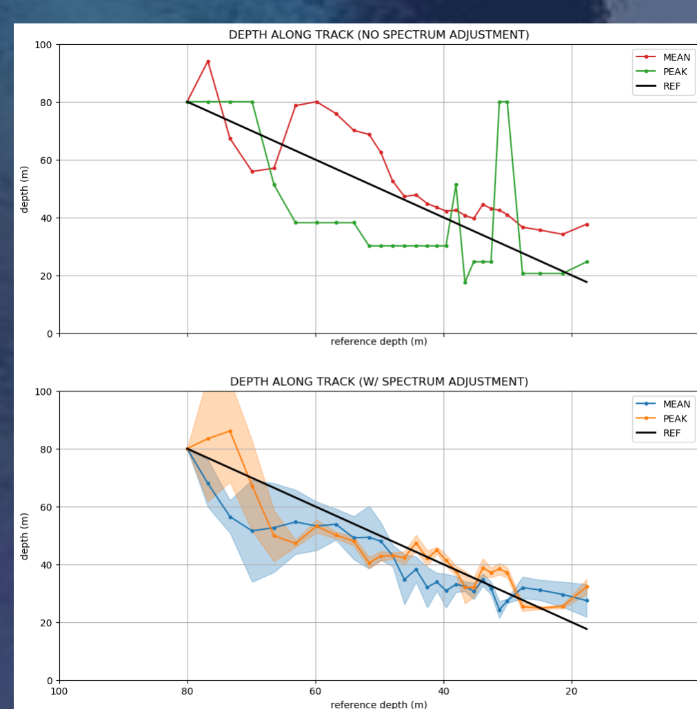
Figure 3: Example of the bathymetry estimated along one single wave ray, with (bottom) and without (top) the spectrum adjustment. The black line represents the reference bathymetry [3] along that wave ray.
