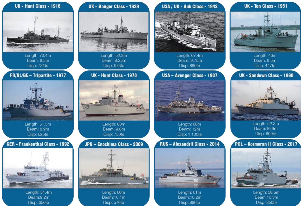
Figure 5 – A selection of Mine Warfare Vessels past and present. These images, and their associated dimensions, show that MCM vessels have not departed far from a common layout and size over the past 100 years. Autonomous technology and developing doctrine is likely to disrupt this trend, leading to a new breed of MCM platform to counter the developing mine threat.
