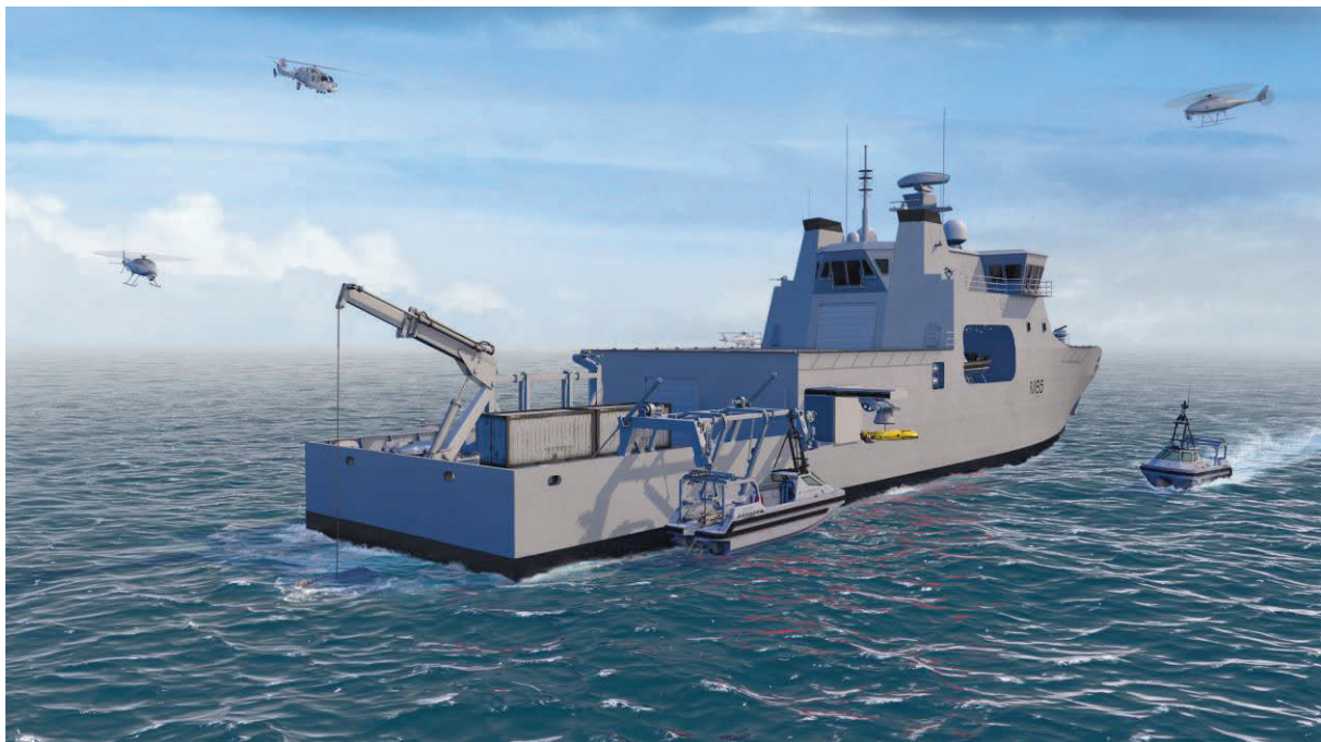
Figure B1 – Indicative arrangement of the new breed of MCM Platform (Image © BMT 2018)
