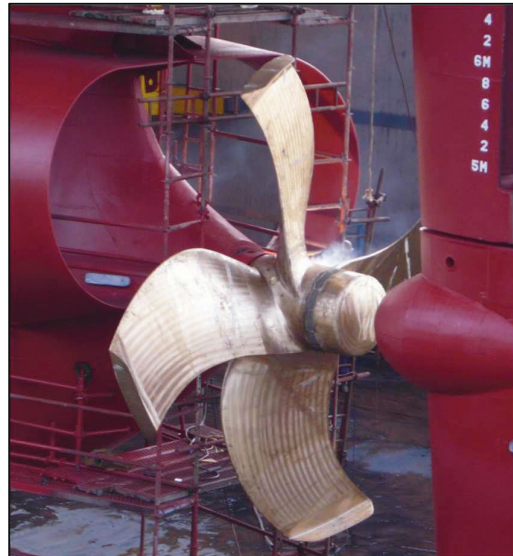
Figure 1 – A contracted loaded tip propeller on a 35000DWT tanker (Gennaro and Gonzales-Adalid, 2012)
