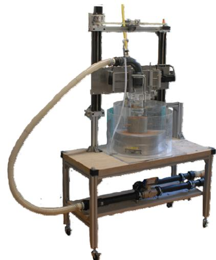
FIGURE 5: L'ESSAI D'ÉROSION PAR JET DE GEOPHYCONSULT
