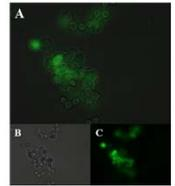
Permeabilized cells: 300ns, ~1.1 MV/m, 20 pulse, 1 Hz = 90% Irreversible EP
