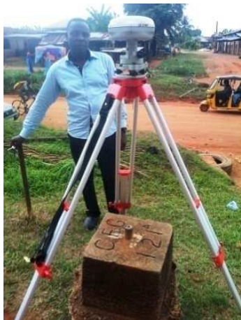
Fig. 3: Base Receiver at Control Station CFG 121 A .
