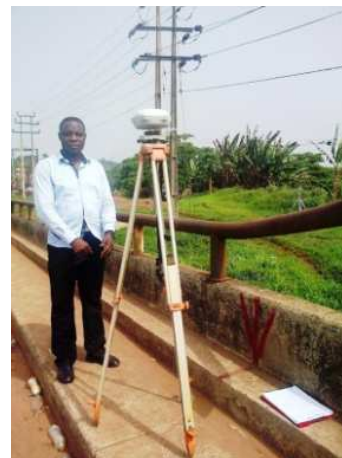
Fig. 5: Rover Receiver at One of the Monitoring Stations on the bridge.
