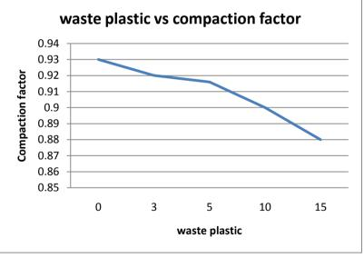
Figure 3: Showing compaction factor values for different percentage of plastic Work Ability by Vee – Bee Consistometer:
