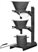
Figure: Compacting factor apparatus
