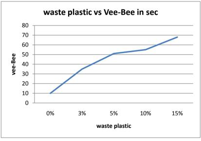
Figure 5: Vee-Bee timing in seconds for different percentage of waste plastic
