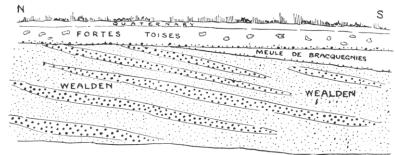
FIG. 13.—Section of Sandpit at Chateau de St. Pierre. (For an account of the beds see the *Geology of Belgium*, pp. 31-2.) Lotice the overlap of the Fortes Toises. The Meule de Bracquenies is ve
