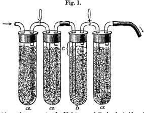
Absorption apparatus for Moisture and Carbonic Acid,  $\times \frac{1}{2}$ . a. Tubes filled with pumice soaked in sulphuric acid. b. Tube filled with soda-lime. c. Plug of cotton wool.
