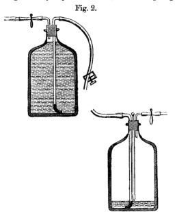
tubing provided with a screw-clip for regulating the rate of aspiration. The burette clips are for starting or stopping the flow. The bottles are covered outside with a layer of felt, to keep the temperature of the air and water equal during an experiment, and also to prevent breakage. A vertical strip on each bottle is, however, left uncovered, so that the height of the water may be watched during the experiment and the
