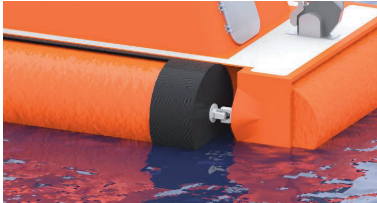
Figure 6 - Indicative concept of HiCEL connection between the expansion shell and the central hull
