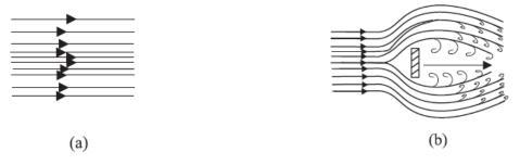
*Fig. 10.8* (a) Some streamlines for fluid flow.(b) A jet of air striking a flat plate placed perpendicular to it. This is an example of turbulent flow.
