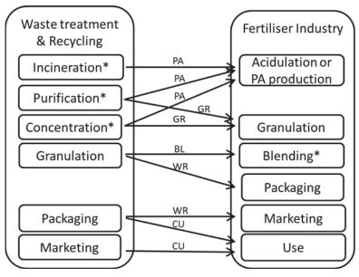
Figure 4: Processes for mineral fertilizer production and marketing. On the one hand from waste and on the other hand in the fertilizer industry from phosphorus rock. Arrows indicate possible entry points in the fertilizer production value chain. Optional processes marked with\*. PA denotes Phosphoric Acid.
