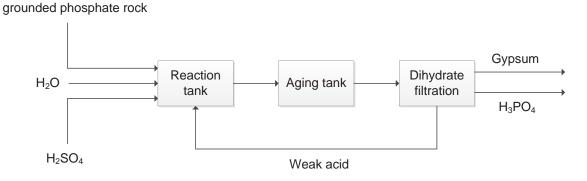
Figure 10: Process scheme of the Dihydrate process (European Commission, 2007)
