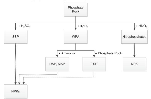
Figure 8: Process scheme for producing different types of fertilizer (International Plant Nutrition Institute , 2010)
