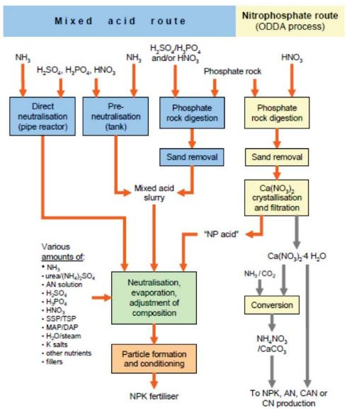
Figure 9: Overview of the production of NPK fertilisers from phosphate rock or SSP/TSP (European Commission, 2007)
