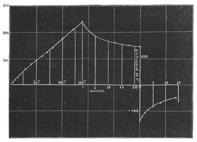
the first part of the curve the ordinates are the scale-readings, the abscissæ the angle turned through by the torsion-head,
